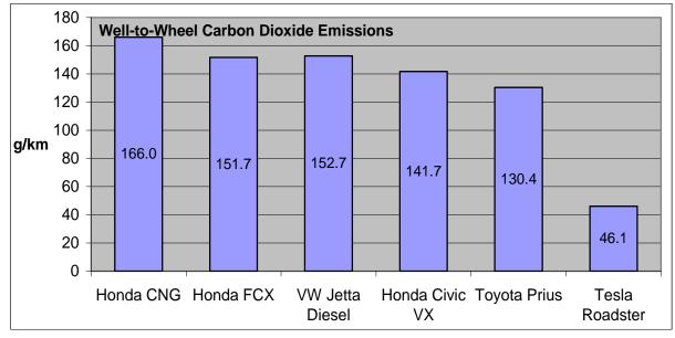
Again, the electric car shines – from the perspective of  $CO_2$  emissions, it is three times better than the hybrid car, and nearly four times better than the hydrogen fuel-cell car.
