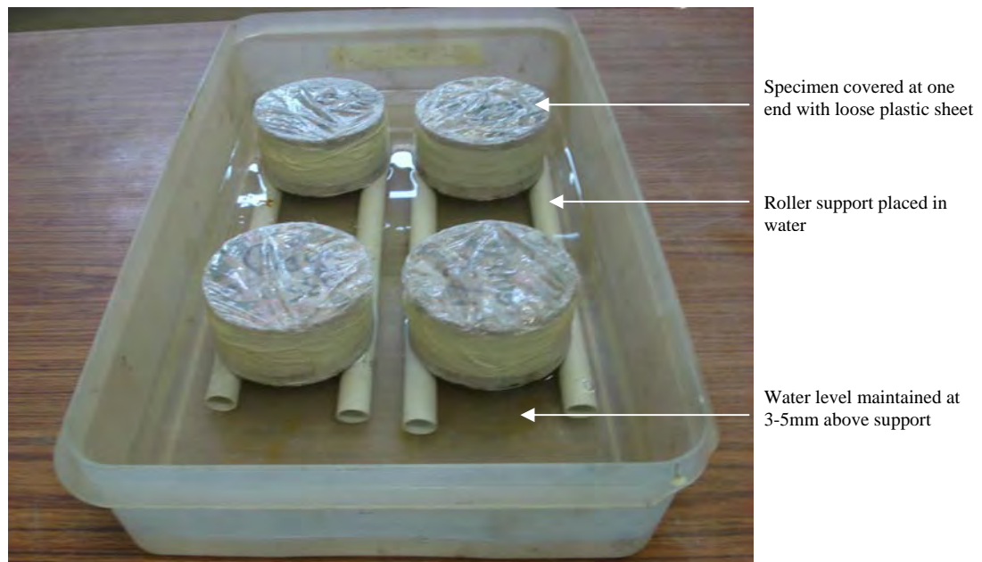
Figure 1: A typical sorptivity test set-up
