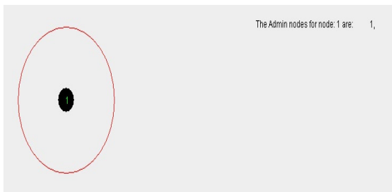
Figure 3: The first node on entering the network broadcasts a hello packet within its range. But as it gets no response it does not flood its neighbor list. It is its own admin
