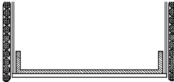
Fig. 12 Structure of load for induction heater using single metallic sheet
